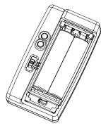
Open the battery cover. Then, set the slide switch to **Setup**.
