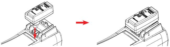
Snap the optic side of the U1177A to the multimeter IR communication port.
